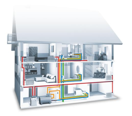
ArmaLight Tubolit saves energy, improves acoustic comfort in buildings and protects pipes installed within the building shell. ArmaLight Tubolit is the most complete range of thermal, acoustical and protective insulation products for installations of heating, domestic hot and cold water and sewage pipes in both residential as well as public and commercial buildings.
